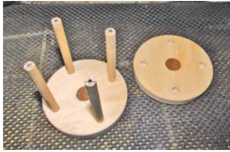
▲ Pic.8 Glue the columns into one of the wheels only, dry-fitting the other to apply pressure
